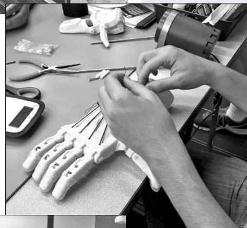
[CENTER] Working with the 3D-printed prosthetic hand, CADD students are installing the cables that allow the fingers to return to a natural position
