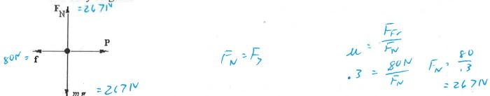
$\mathbf{F}_{N}$  represents the normal force on the block; and  $\mathbf{f}$  represents the force of kinetic friction.
